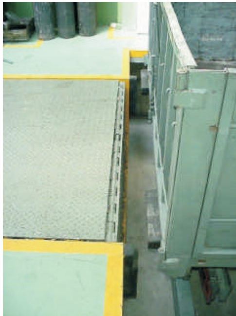
Leveller fully lowered in rest position - lip in "keepers"
