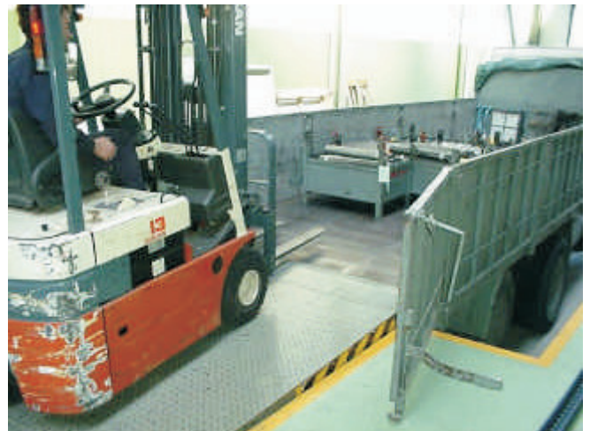
Leveller floating on truck - ready for un-loading by fork-lift truck
