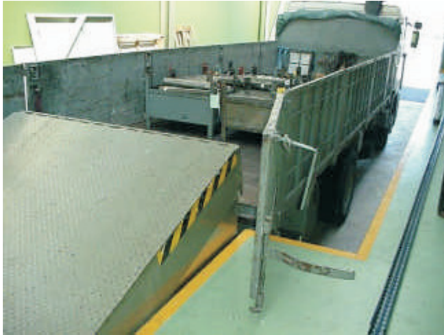
Leveller rising (lip falls automatically)
